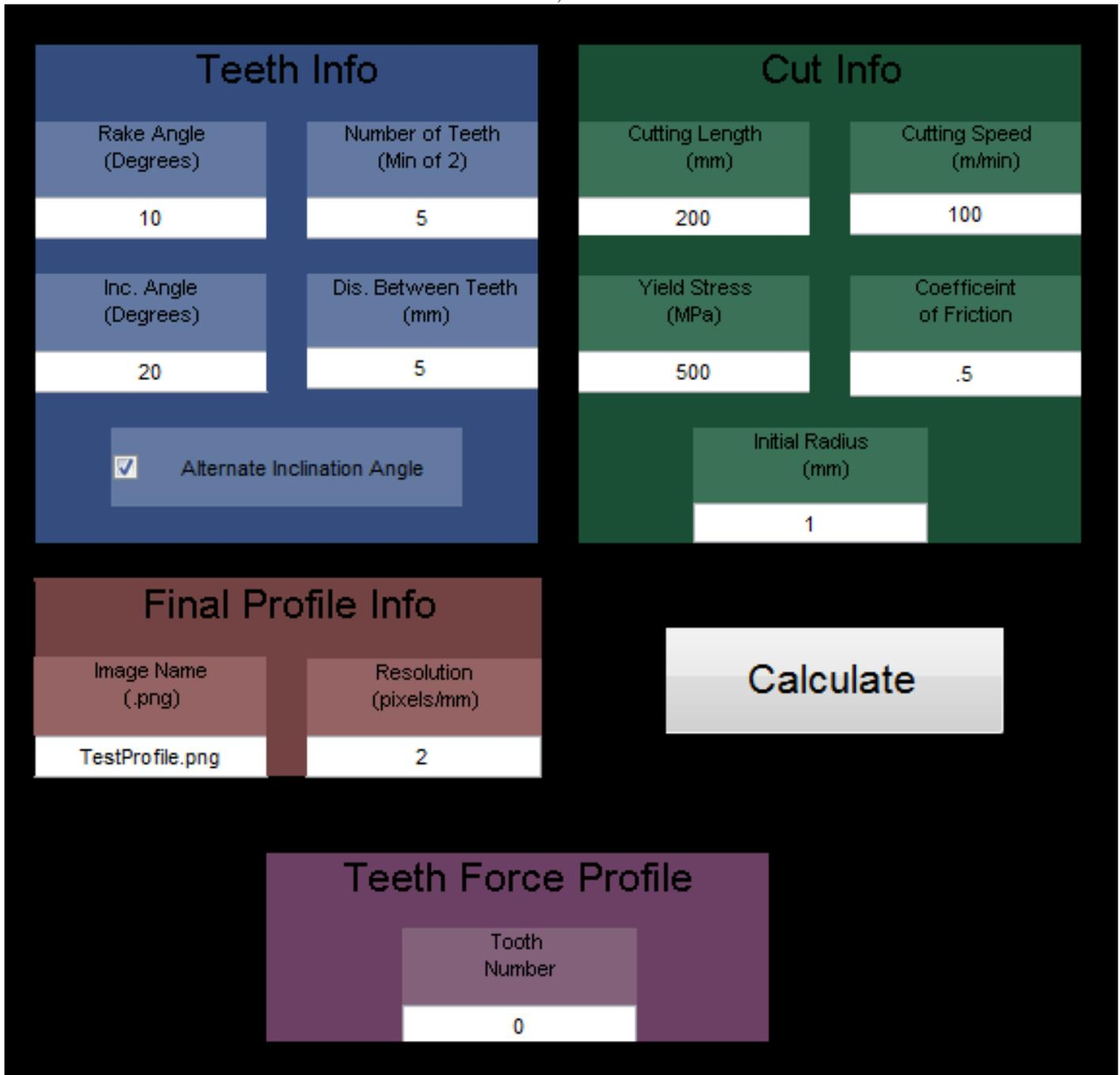
Figure C3: The GUI can control various parameters about the teeth (blue section) as well as parameters about the cut and workpiece (green). In addition, the user can specify the image file and resolution being used for the final tooth profile (brown). Finally, if the user desires, they can bring up the force profiles for a specific tooth in the broaching tool (purple).
